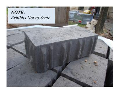
PERMEABLE PAVERS MIN. 3 1/8" (80mm) THICK
